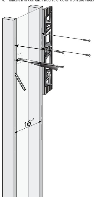
**Note:** The top of the unit must be installed a minimum of 6" and a maximum of 18" from the ceiling.
