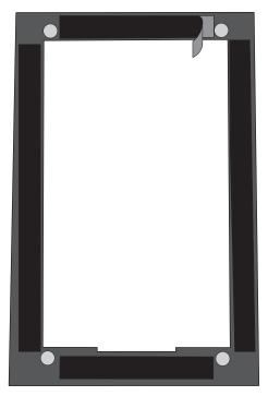
6. Align magnets with previously drilled holes. Make sure the cut-out portion of the bracket (circled below) is on the bottom. Press the bracket firmly against the wall.
