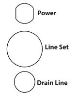
6. Depending on the desired installation, remove the rear or bottom knockouts for the line set, drain line, and power cord.
