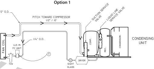
SINGLE FAN COIL PIPING SYSTEM
