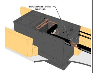
13. Braze the copper tubing to the connections on the evaporator unit.
