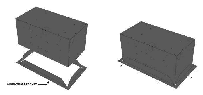
4. Secure the unit's mounting bracket to the opening using the twelve (12) supplied 2½" Phillips-head screws.
