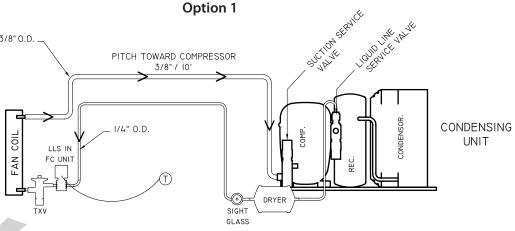
SINGLE FAN COIL PIPING SYSTEM
