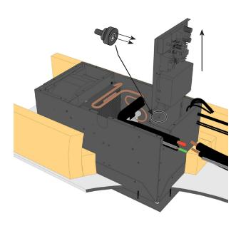
17. Slide the electrical panel up and out of the unit.
