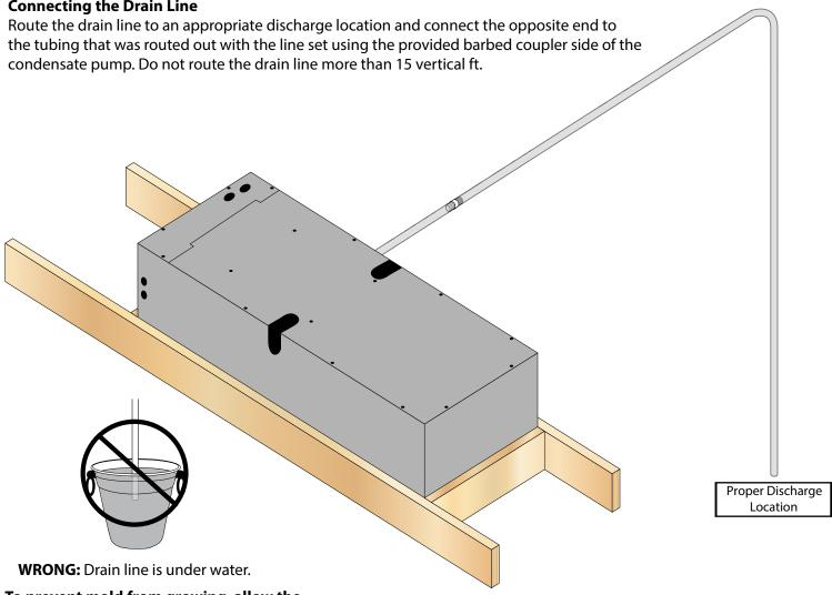
To prevent mold from growing, allow the drain line to hang above the water line.
