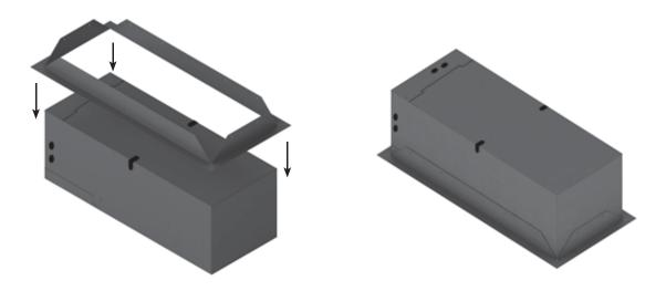
4. Secure the unit's mounting bracket to the opening using the twelve (12) supplied 2½" Phillips-head screws.
