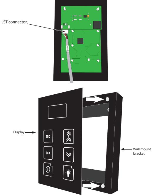
5. Place the display on the wall mount bracket as shown, attaching the back of the display panel to the magnets on the mounting bracket. Make sure that the alignment tab on the back of the display panel sits in the notch on the bottom of the bracket.
