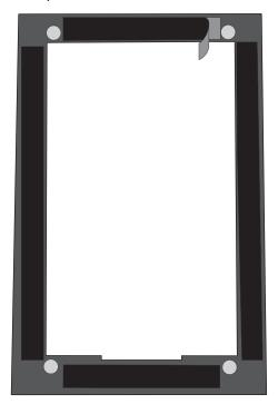
6. Align magnets with previously drilled holes. Make sure the cut-out portion of the bracket (circled below) is on the bottom. Press the bracket firmly against the wall.
