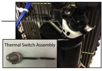
Slide the thermal switch to the location shown
