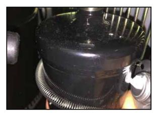
Set thermal switch in location shown, making sure the surface of the switch is making good contact with the receiver.
