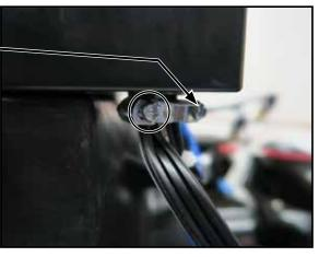
Route the two long white wires from the silicone heaters up into the electrical box.
