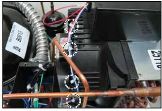
Zip tie the wires going into the N1 and H1 lever connectors as shown.
