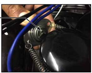
Secure the white wires from the heaters to the - lever connector labeled **N2**.
