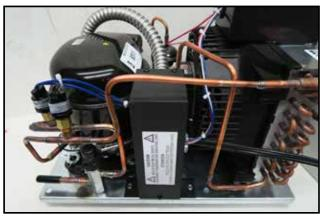
Cut and remove the zip tie holding the fan and ground wires to the capacitor bracket on the compressor.
