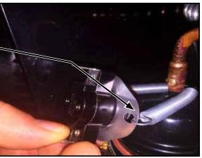
Slide the thermal switch to the location shown. Make sure the tab of the thermal switch rests on the screw terminal of the top hose clamp.
