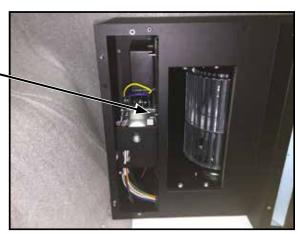
Re-install the electrical panel using the 2 Phillips head screws removed in step #6.
