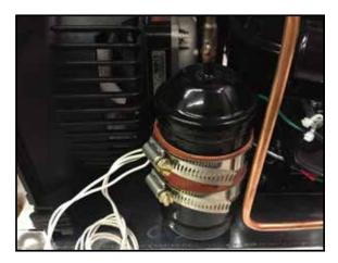
Wrap the spring from the thermal switch around the liquid line and secure the clasp of the spring to the thermal switch as shown.
