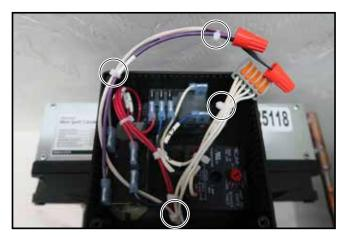
Secure the Cold Weather Start Kit box to the top of the coil using the ½" self taping screws provided. (Using screws or mounting locations other than the ones specified, may result in a punctured coil.)
