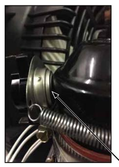
**NOTE**: Make sure the surface of the thermal switch is located at the ridge of the receiver, - and is making good contact.
