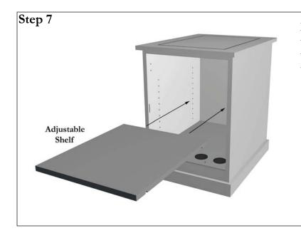
Locate the adjustable shelf and four shelf pins. Insert the shelf pins in the chosen location. Set the shelf on top of the shelf pins so that it rests in the groove on the bottom of the shelf.
