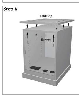
Locate the tabletop and place over the top of the humidor. The groove on the bottom side of the tabletop fits right over the top of the humidor. Secure in place with the six round head washer screws provided.
