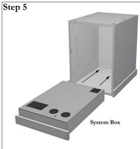
Note: If you purchased a System upgrade, you will need to place the lower hinge in place before sliding your system box into the cabinet. Please view steps 1-2 under the door installation steps on page 5.
