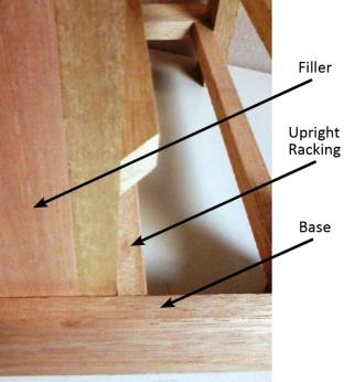
Figure 66: Faceframe with Racking
