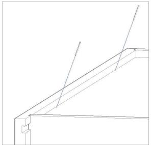
Figure 57: Brad Back Panel into Side Panels
