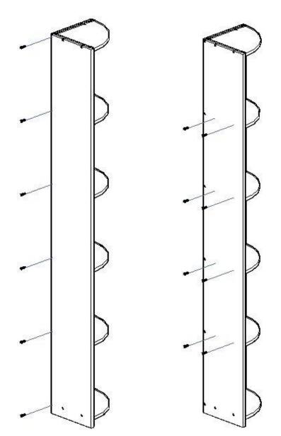
Figure 46: Affix Side Panel to Back Panel along Spine and Affix Shelves to Side and Back Panels
