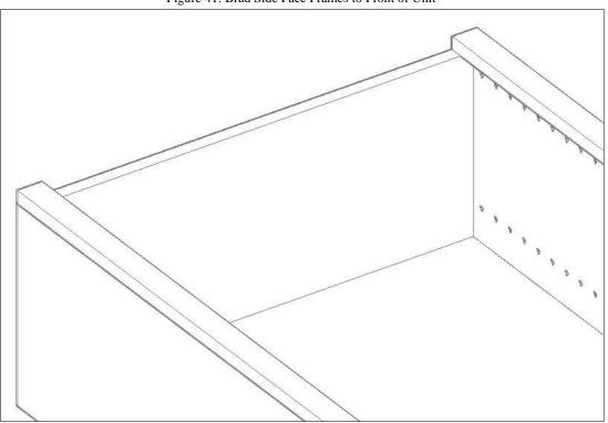
Figure 41: Brad Side Face Frames to Front of Unit
