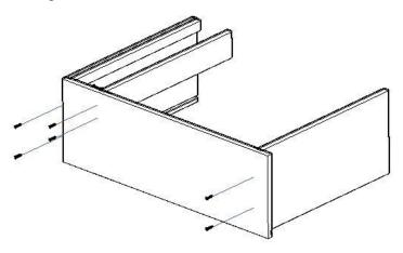
Figure 54Figure 54: Affix Stretcher to Top and Bottom Panels
